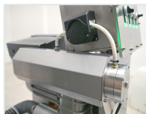
Solution system with hose pump feeding directly from any external container
